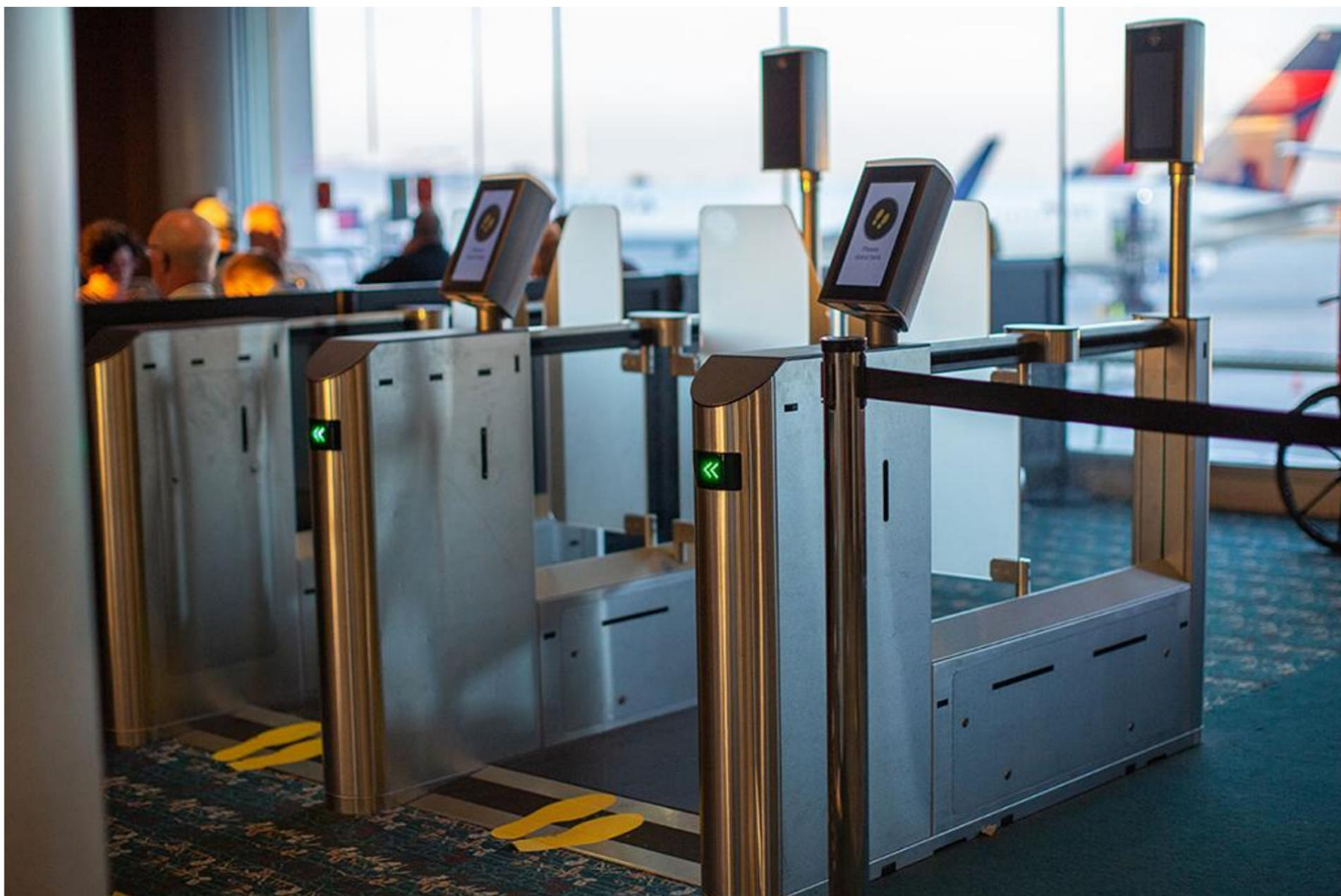
The SITA SmartPath automated boarding gate uses facial biometrics as proof of identity, eliminating the need to produce a boarding pass. Credit: SITA
