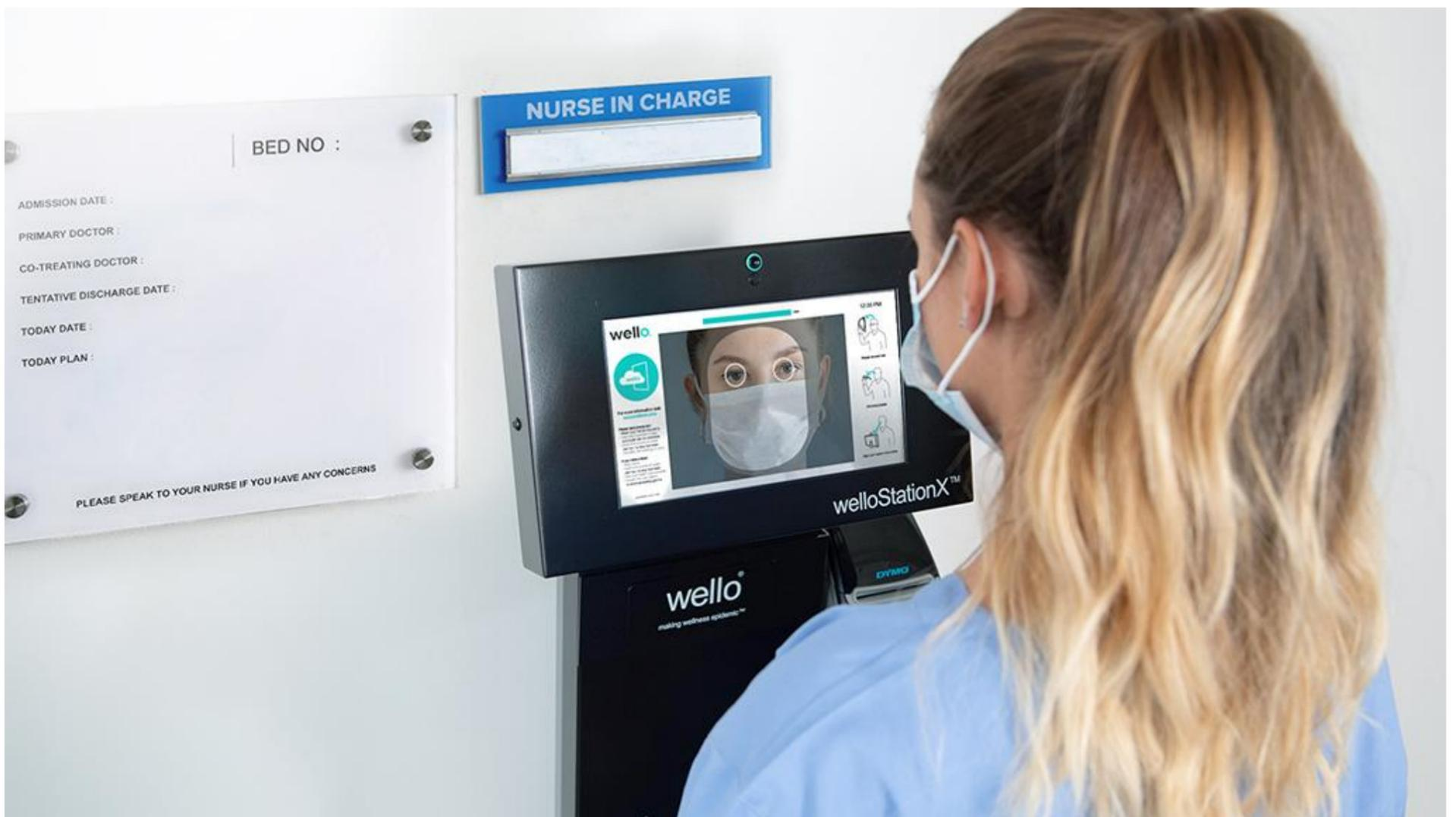
The welloStationX is an automated contactless temperature screening system. Credit: Wello
