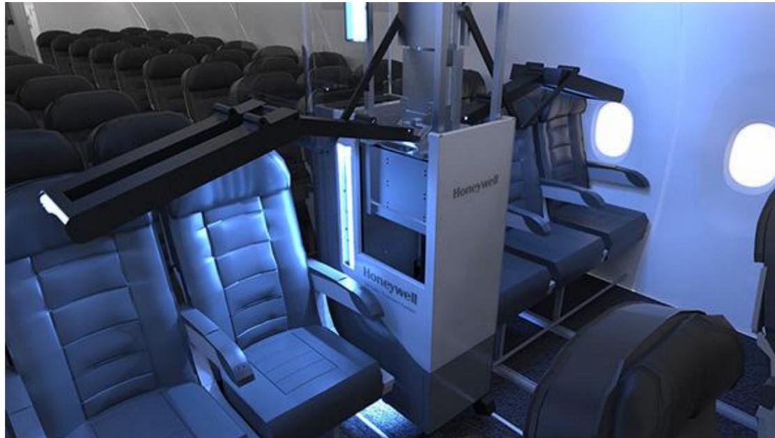
Honeywell's UV Cabin System shines germicidal ultraviolet-C light on interior surfaces.
