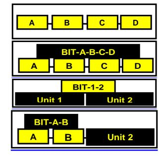
**Legend:** A, B, C, D, Unit1 and Unit2 are Line Replaceable Units and BIT is Built-In-Test devise that identifies a failed LRU.
